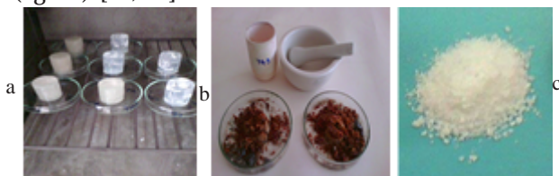
Fig. 1. The steps of obtaining sol-gel glasses: a - aged gels, b - xerogels \text{Ag}^+ , c - bioglass powder
